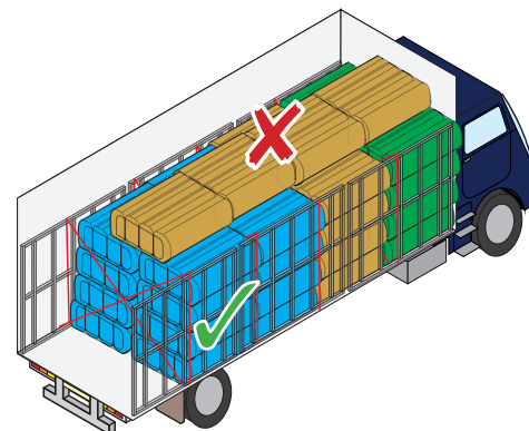
Gates are braced but product is loaded above the top of the gate with no tie down restraint
