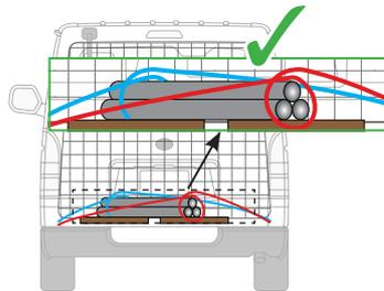
Thin items should be loaded diagonally and secured to the floor with belly wraps.
