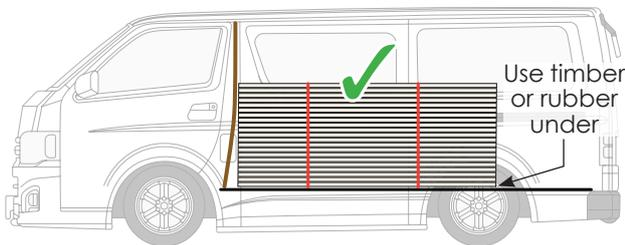
Heavier loads need to be tied down. Use rubber or timber under the load and aim to block forwards.
