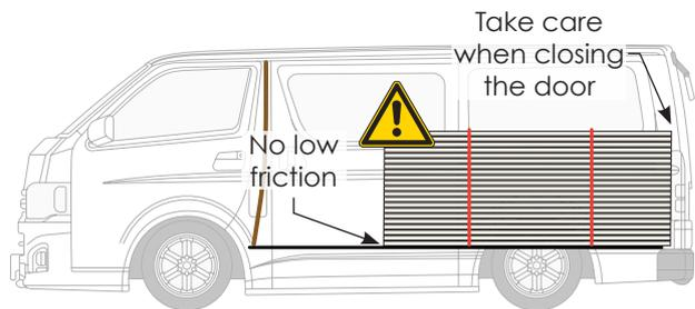
Avoid gaps. Where a gap is essential, tie the load down. Always load on rubber or timber.
