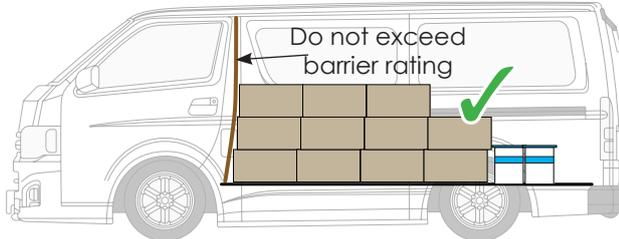
Distribute the load along the van, starting from the front blocked against the cargo barrier. Do not exceed manufactures rating for loose loads.
