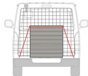
Secure heavy loads centrally across the vehicle with rubber or timber under the load.
