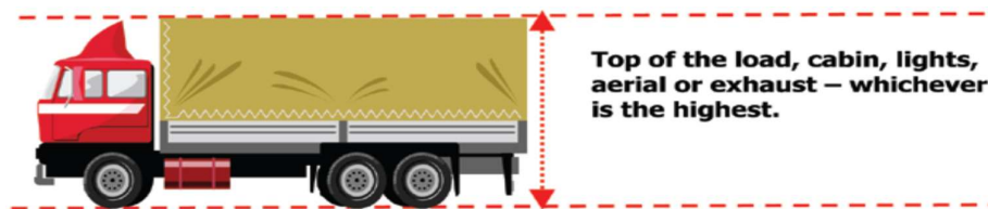
Figure 8 Transit Envelope – The maximum overall height of the vehicle
