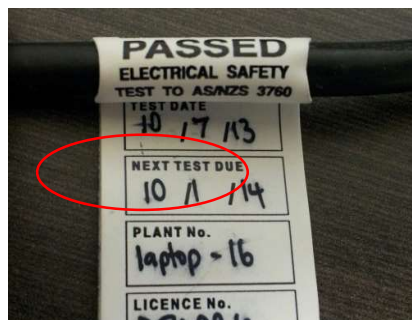
Figure 4 Typical electrical safety test tag with 'Next test due' date circled
