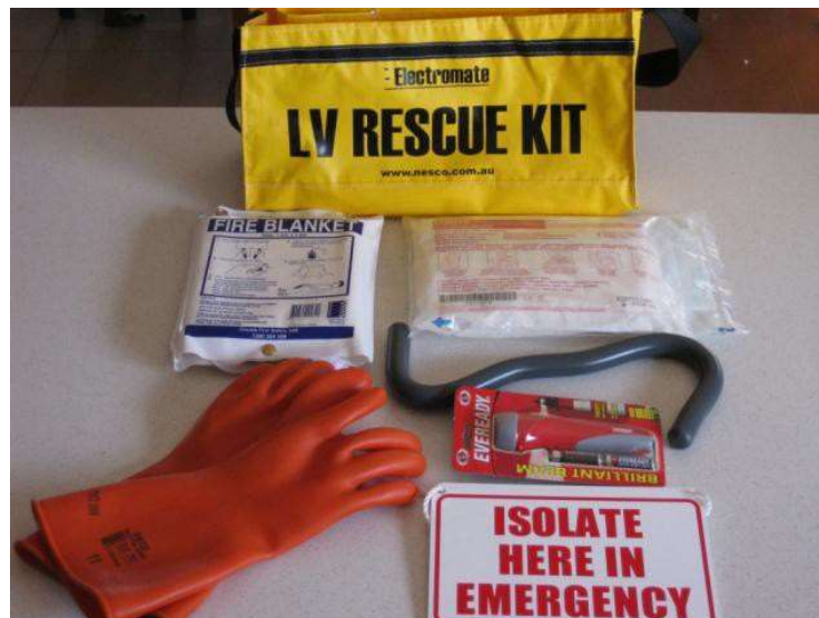
Figure 14 Low voltage rescue kit contents
