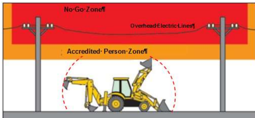
Figure 11 Consideration of Mobile Plant Vertical Operating Envelope
